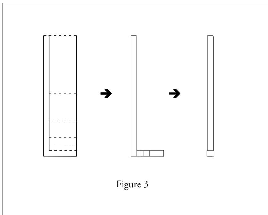
As a result, we obtained essentially a pendulum analog having the same mass as the electroscopic leaf, but with nearly 90% of its mass concentrated near the tip, while retaining perfectly continuous conductivity with the electroscopic stem. We weight-pressed the fashioned pendulum and then tacked the outer leaf fold to the suspension strip with a micro-drop of cyanoacrylate.
