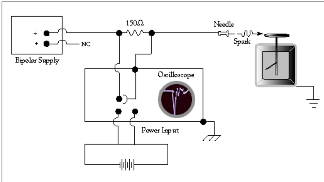
Fig. 2 - Experimental circuit employed to charge and monitor the electrostatic voltmeter.
