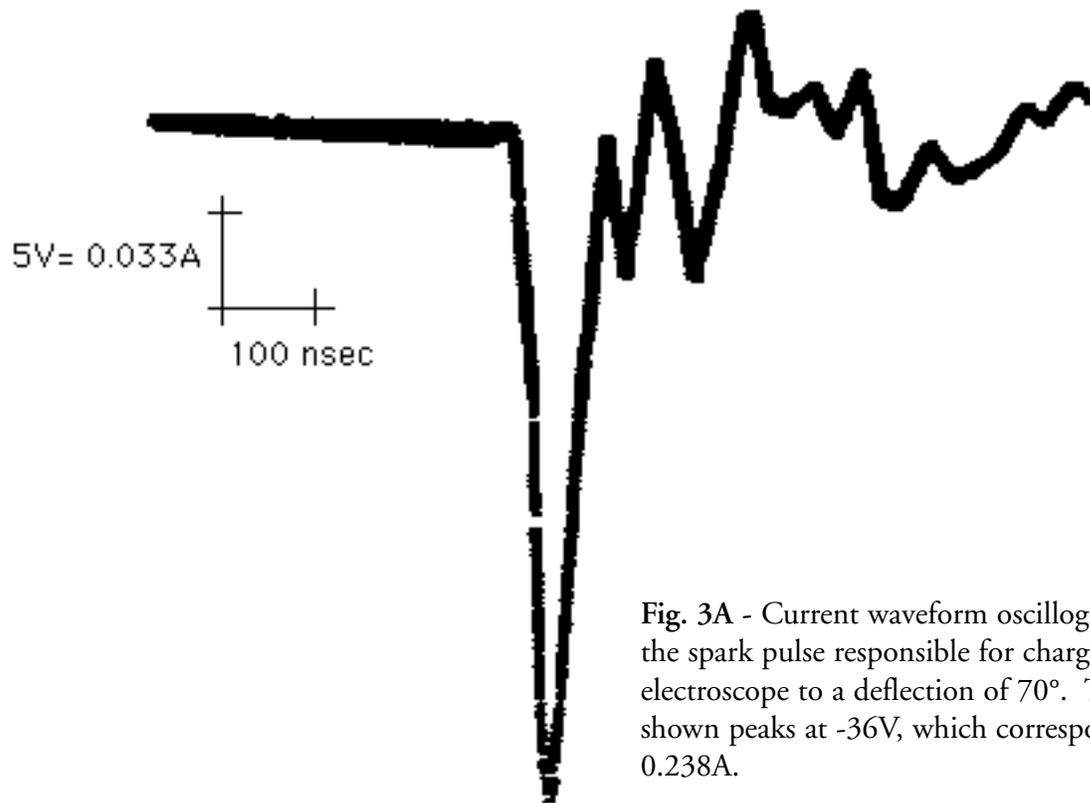
Fig. 3A - Current waveform oscillogram of the spark pulse responsible for charging the electroscope to a deflection of 70°. The pulse shown peaks at -36V, which corresponds to 0.238A.
