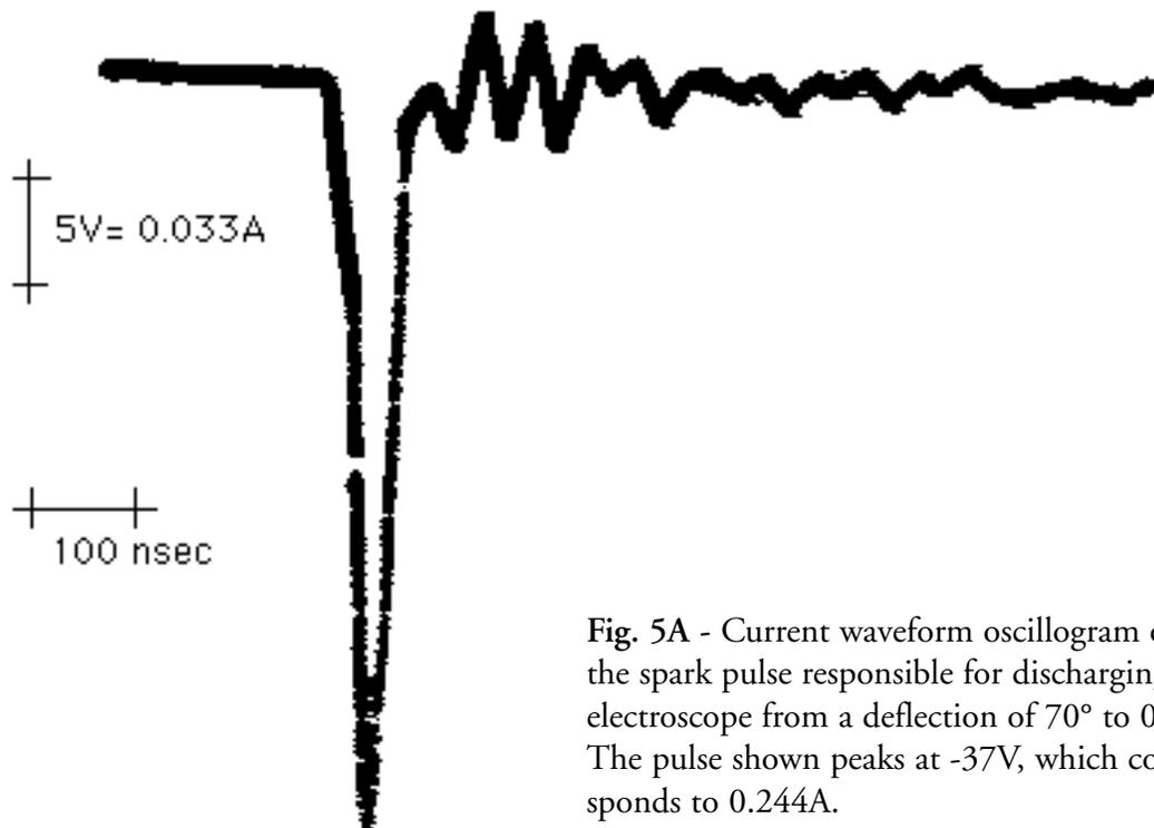
Fig. 5A - Current waveform oscillogram of the spark pulse responsible for discharging the electroscop from a deflection of  $70^\circ$  to  $0^\circ$ . The pulse shown peaks at  $-37V$ , which corresponds to  $0.244A$ .
