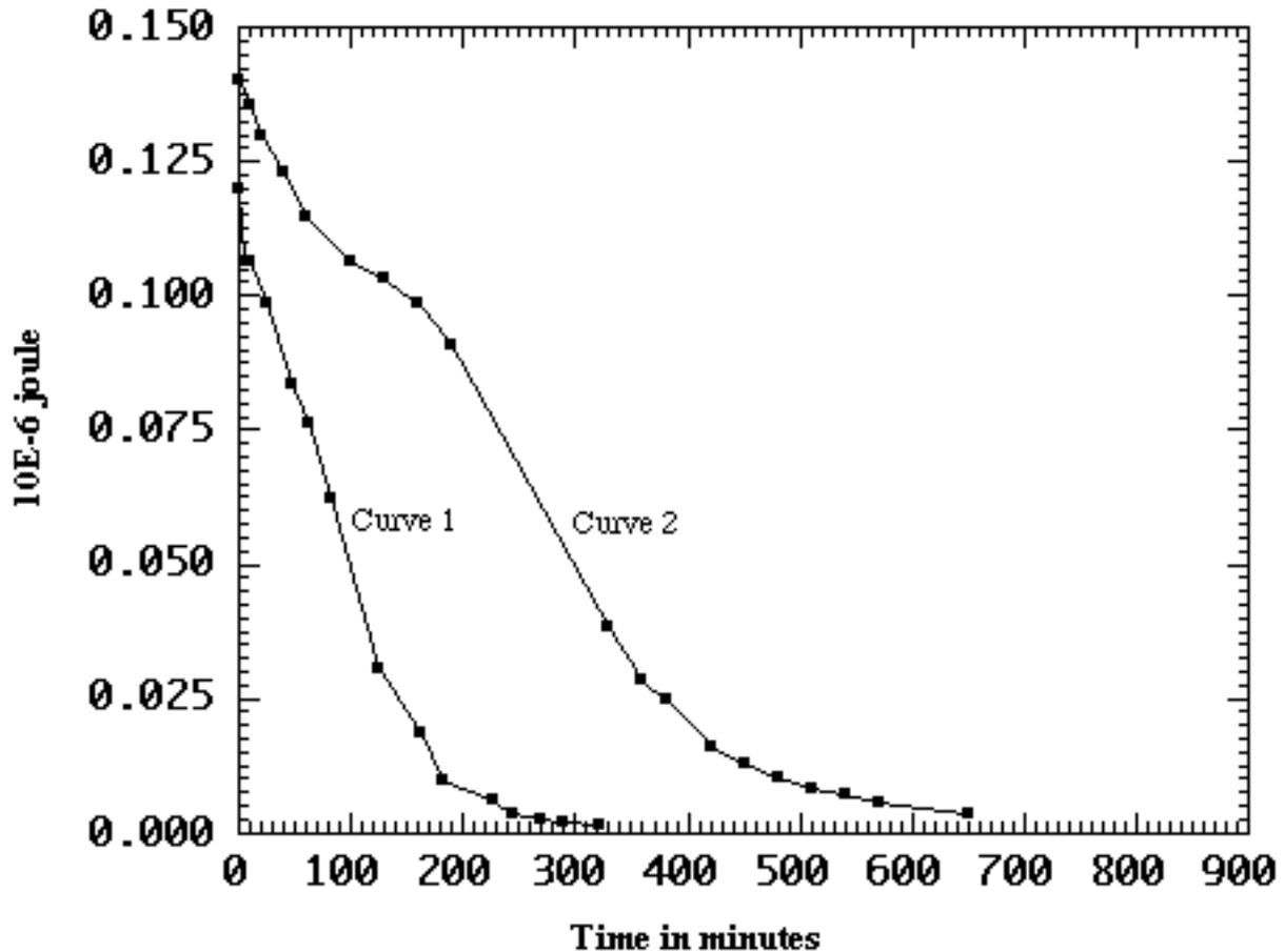
Fig. 6 - Variation of free leakage moment (joule-sec) as work-equivalent positional energy over time, for the same negatively charged electroscope under widely different atmospheric conditions. Initial electroscopic deflection: 70°.
