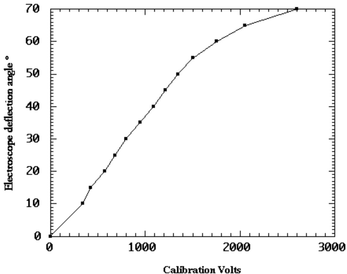
Fig. 1 - Calibration curve of the gold-leaf electroscope with a negative voltage supply.
