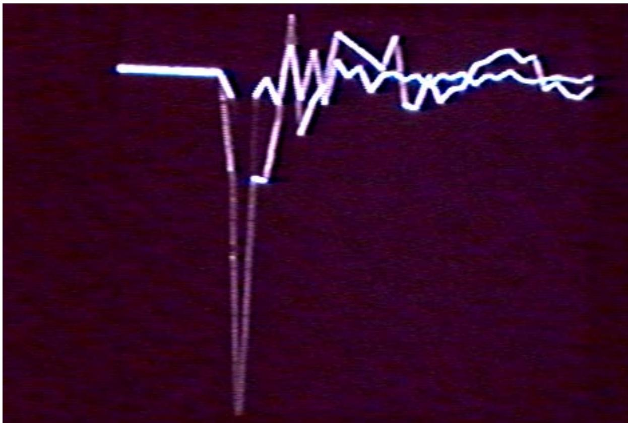
Fig. 5B - Juxtaposition of input and output current pulses, to and from the electroscop. Start or end-point deflection, respectively, for the output and input pulses, was  $70^\circ$ . The input pulse is that shown in Fig. 3A, and the output pulse, that shown in Fig. 5A.
