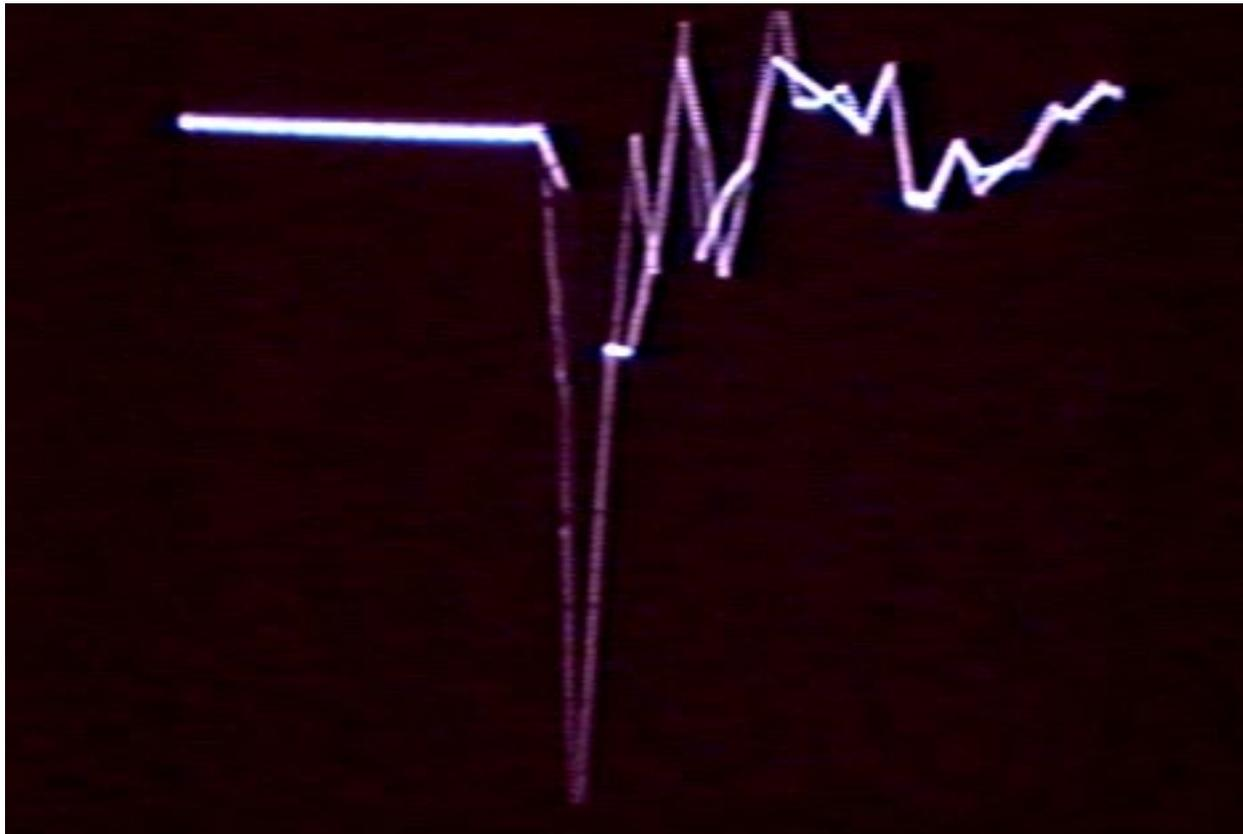
Fig. 3B - Juxtaposition of two input current pulses charging the electroscope to a deflection of 70°. X: 100nsec/div; Y: 5V/div
