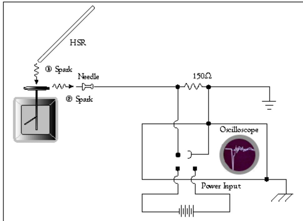
Fig. 4 - Experimental circuit employed to discharge and monitor the electrostatic discharge.
