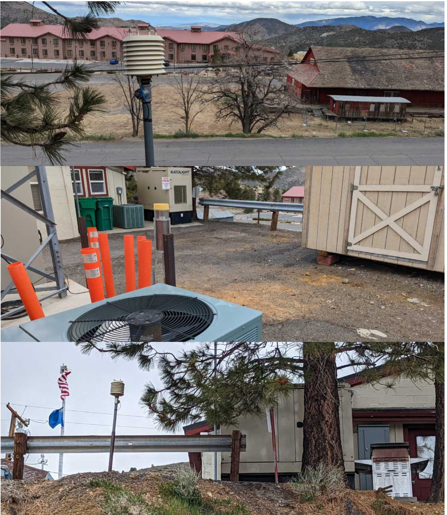
MMTS placement at the Storey County Volunteer Fire Department in Virginia City, NV. This is a GHCN station with records dating back to 1887. Note in the close-up photo, the top solar shield cap of the MMTS is missing. Multiple heat sinks are in proximity to the sensor, including asphalt, concrete, a barbecue grill, two a/c units, a generator, and multiple structures providing wind sheltering. Source: Anthony Watts.
