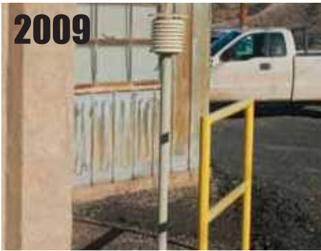
Miami, AZ , sited on dark gravel, next to building. RATING = CRN5
