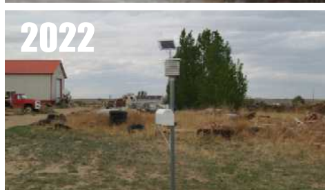
Moved, but new station is compromised by addition of mailbox and solar panel. RATING = indeterminate, there is no formula for mailboxes.
