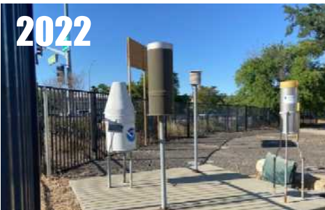
Location unchanged, but wooden slat/chain-link fence to the north has been removed. RATING = CRN5
