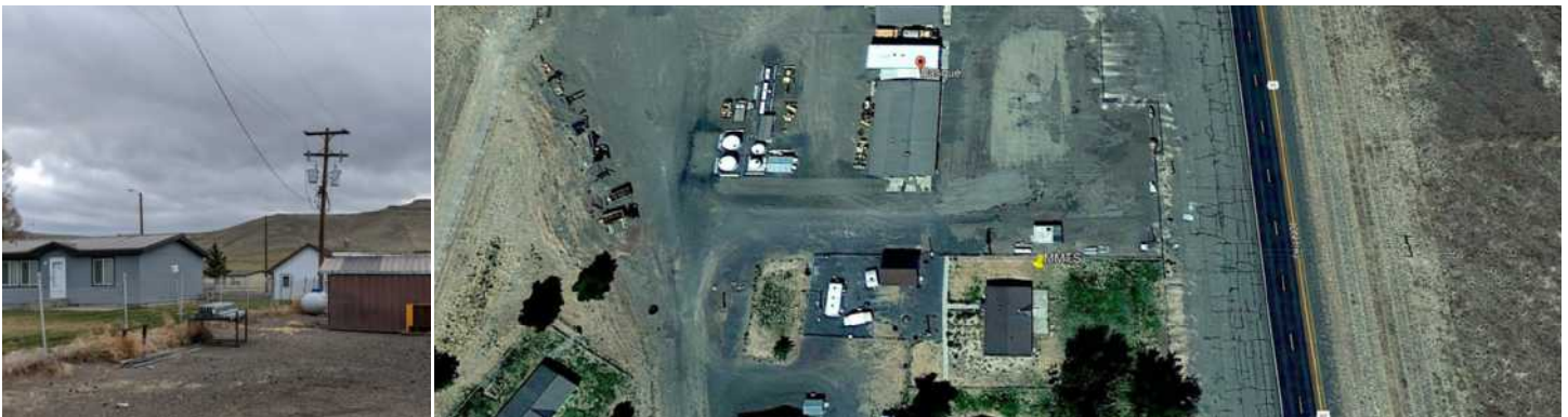
MMTS placement in COOP observer's yard next to an ODOT maintenance facility in Basque, OR. Note the very large asphalt parking lot in the aerial photo and the yellow marker indicating the MMTS placement. Basque is an isolated small town, with the next town 30 miles away. It would be categorized as exceptionally rural, yet the GHCN thermometer is placed directly next to the largest heat sink. Source: Anthony Watts, Google Earth.
