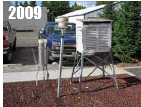
Waterville, WA , over cinder rock, adjacent to sidewalk, parking lot. RATING = CRN5
