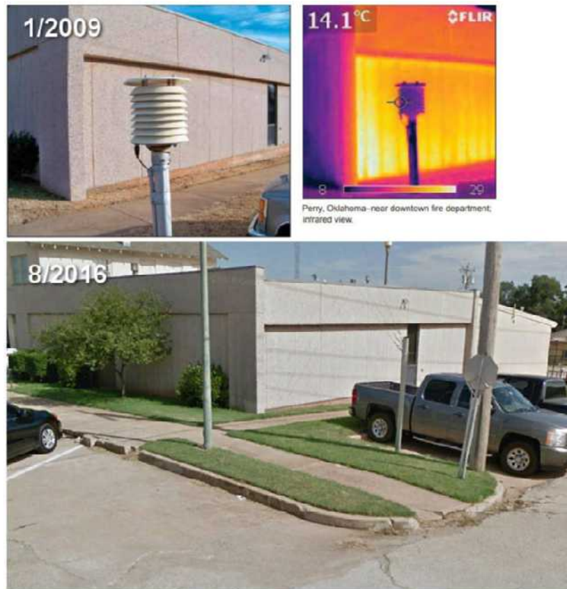
Figure 10: Before and after photographs of the Perry, OK, USHCN station. Top: natural and infrared photos indicating heat effects of building wall in January 2009. Bottom: Perry, OK, street view from August 2016. Source: Anthony Watts, Google Earth.
