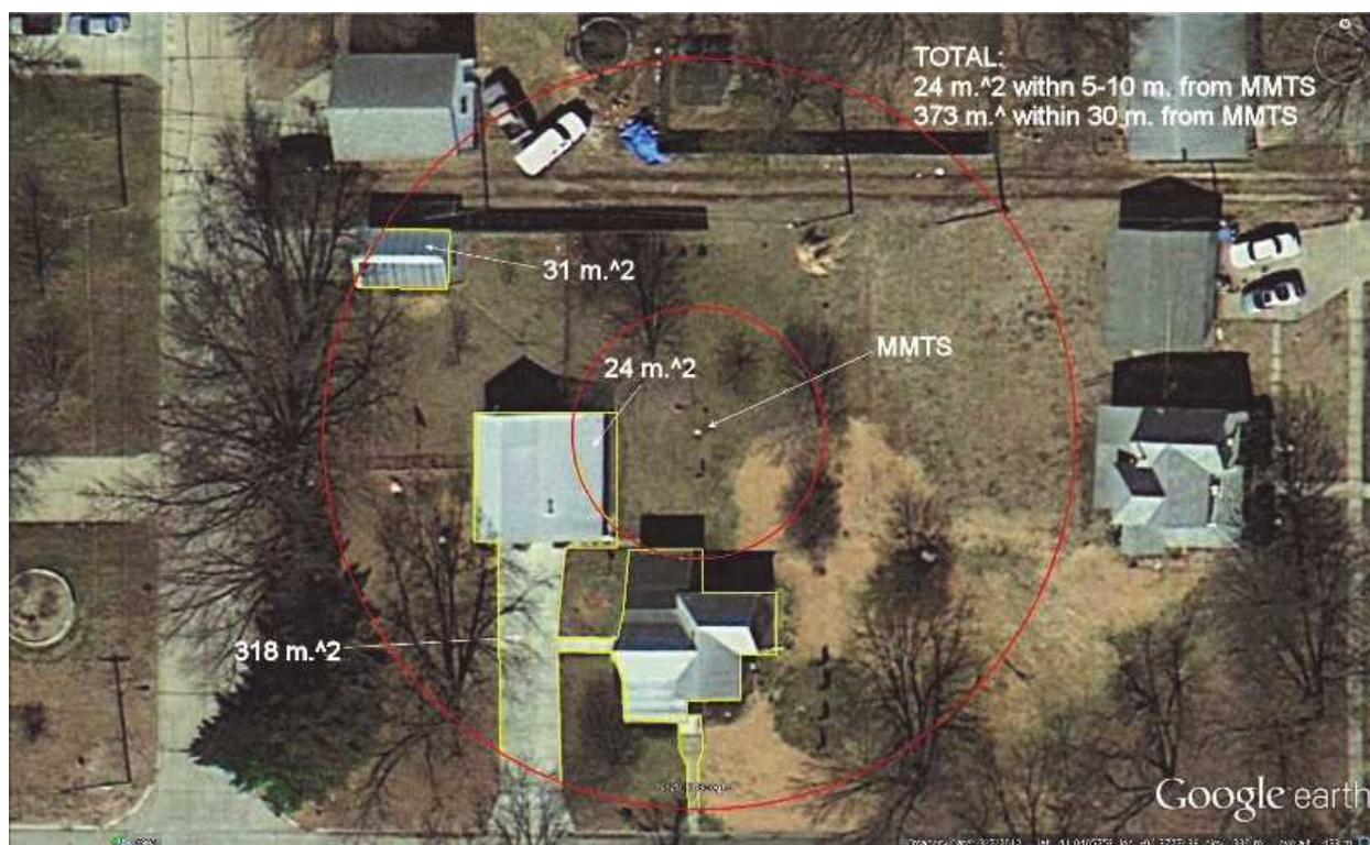
Figure 12: Analysis of artificial surface areas within 10- and 30-meter radii at Ashland, NE, USHCN station (COOP# 250375) using Google Earth tools. The NOAA temperature sensor is labeled as MMTS. The figure illustrates how the USHCN station, which was evaluated per Leroy (2010) procedures, showing the 10- and 30-meter radii, along with polygon surface (area outlines of visible heat sinks created with Google Earth Pro tools, providing a value of approximately 373 square meters of heat sink surface area within the 30-meter radius, and approximately 24 square meters within the 5-10-meter annulus). Source: Anthony Watts and Evan Jones.
