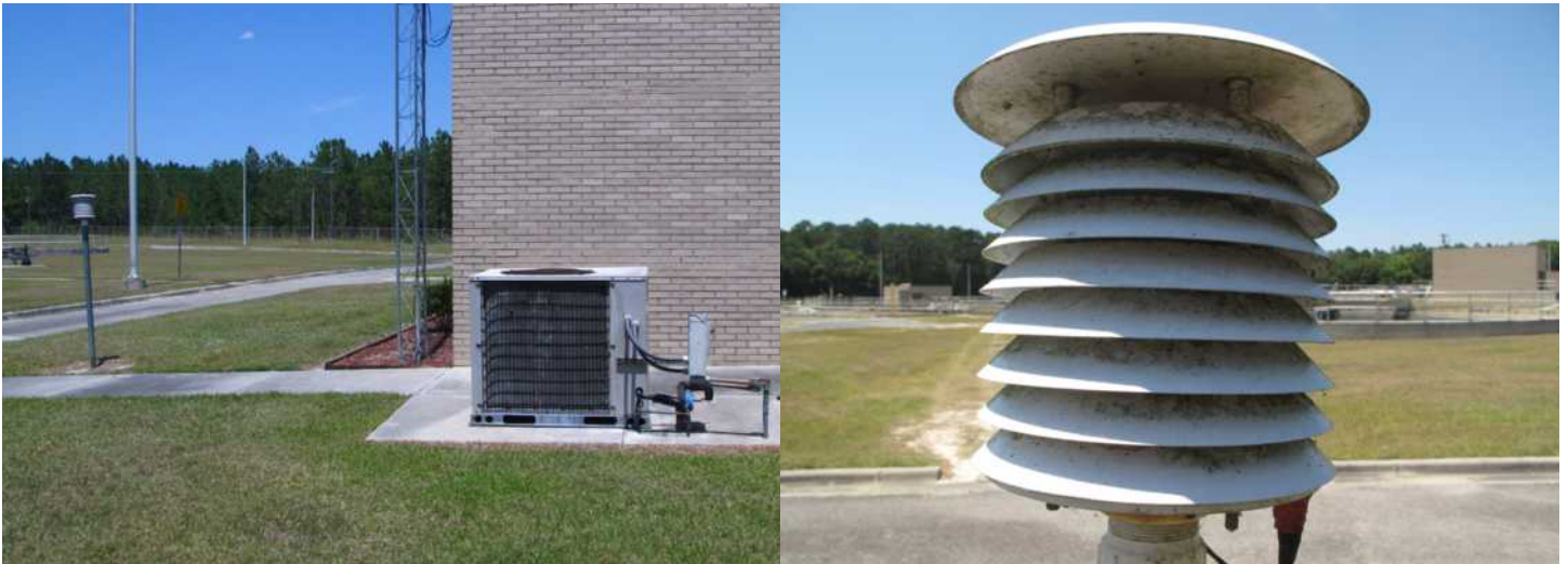
USHCN station at WWTP in Tifton, GA. Note the MMTS is directly over a sidewalk, near a brick wall, and near a/c units. This is a Class 5 station. Note in the second photo the discoloration of the MMTS, making it darker, prone to absorb more sunlight, and subsequently warmer. Source: Alan Watt.
