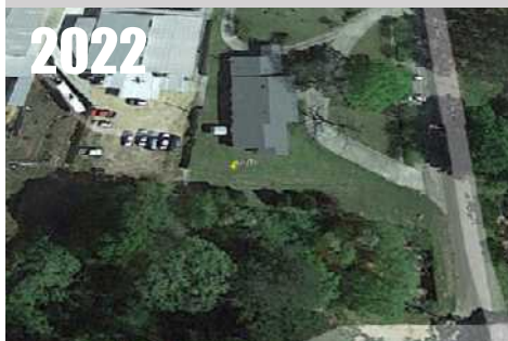
Moved to new location at city offices on lawn. Improved location, but still too close to buildings. RATING = CRN3
