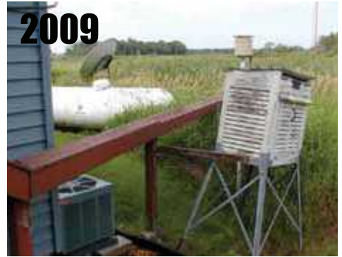
Detroit Lakes, MN. , nearby air-conditioning unit, building, gas tank. RATING = CRN5
