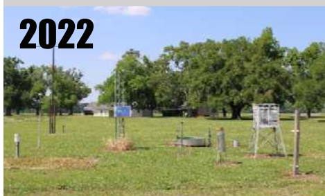
No change. However, CRS is in serious need of maintenance and peeling paint/dirt/missing slats will make it warmer than normal. RATING = CRN1
