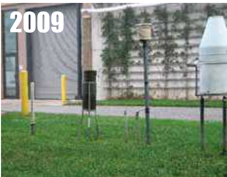
Northfield, VT , nearby driveway, building. RATING = CRN4
