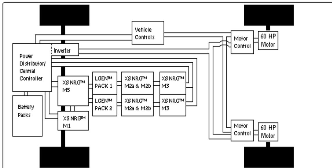
**Fig. 8- Class 1, Type 2 XS NRG™ autonomous electrical vehicle (AEV) utilizing an AC motor system powered from the electrochemical charge storage system by a Controller/Inverter, which is in turn constantly charged by the plasma reactor-based XS NRG™ Power Generation System.**
