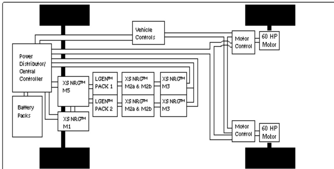
**Fig. 7- Class 1, Type 1 XS NRG™ autonomous electrical vehicle (AEV) utilizing a DC motor system directly powered from the electrochemical charge storage system, which is in turn constantly charged by the plasma reactor-based XS NRG Power Generation System.**
