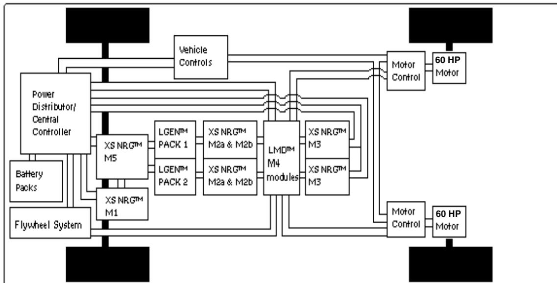
**Fig. 10- Class 3, Type 5 XS NRG™ autonomous electrical vehicle (AEV) utilizing an AC motor system and an AC input flywheel directly powered from the LGEN™ plasma reactors by the LMD modules, which are in turn constantly charged by the battery-driven XS NRG™ Power Generation System.**
