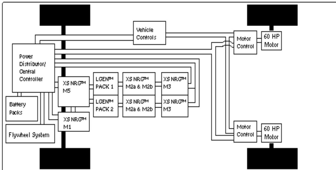
**Fig. 9- Class 2, Type 3 or Type 4 XS NRG™ autonomous electrical vehicle (AEV) utilizing a DC (or AC, not shown) motor system directly powered from the joint electrochemical and flywheel charge storage systems, which are in turn constantly charged by the plasma reactor-based XS NRG™ Power Generation System.**
